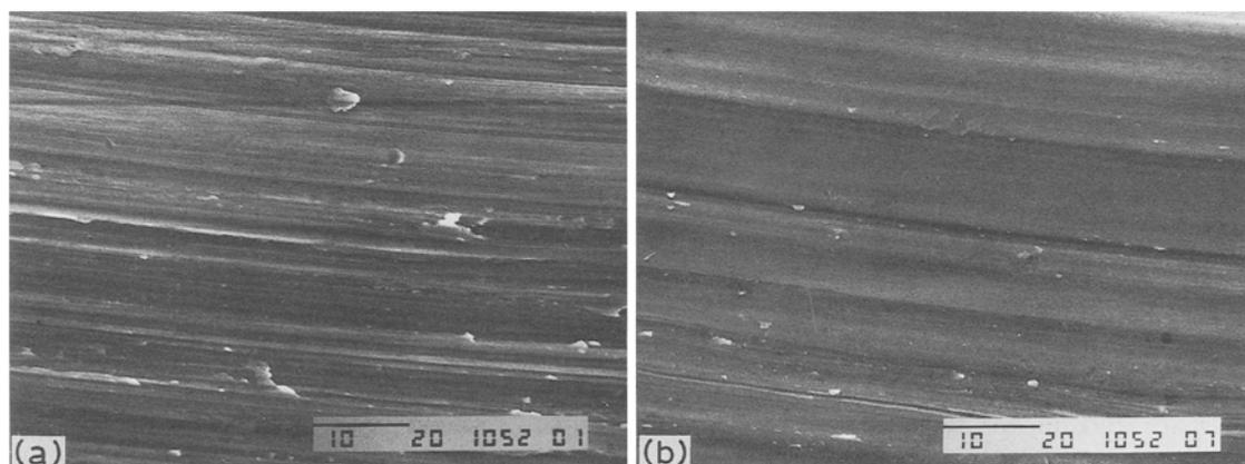
*Figure 2* Scanning electron micrographs of (a) c.p. titanium and (b) Ti-6Al-4V surfaces. The surfaces examined were on the circular plate facing the rod portion of the implant (corresponding to the area used for morphologic analysis). Grooves and ridges, typical for machined metal surfaces, are present on both implant surfaces. Bar = 10  $\mu\text{m}$ .
