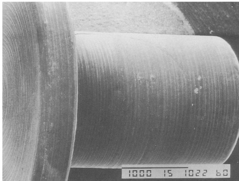
*Figure 1* Scanning electron micrograph of a c.p. titanium implant. The cylindrical rod has a length of 3 mm and a diameter of 2 mm which is connected to the centre of a circular plate that has a thickness of 0.5 mm and a diameter of 4 mm.
